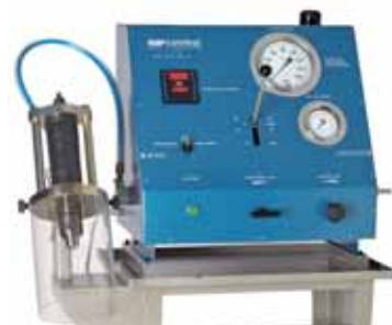
Fuel-injector test rig e.g. IOPmarine (2)
